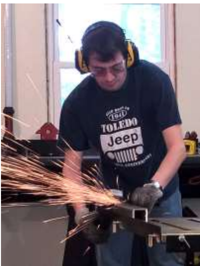
Figure 3: Deburring with angle grinder
