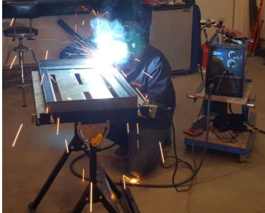
Figure 4: Welding outer frame assembly together
