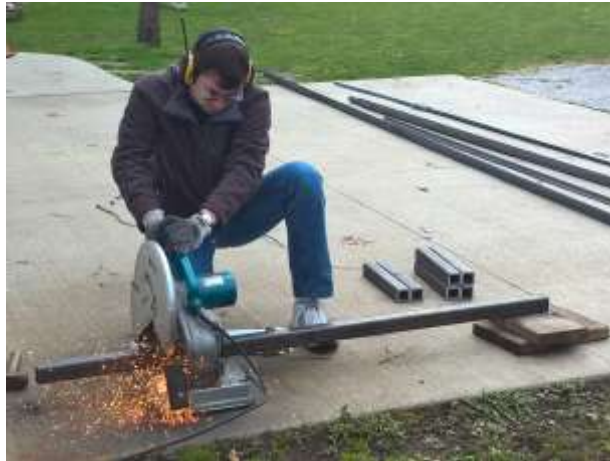
Figure 1: Cutting raw steel to length and proper angles
