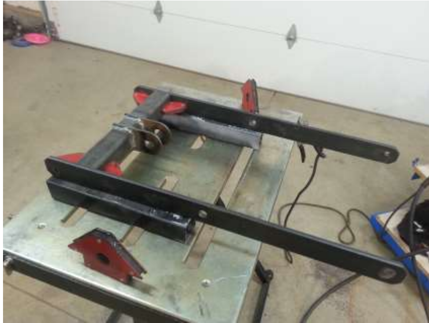
Figure 6: Welding scissor arms to rod end hydraulic mount
